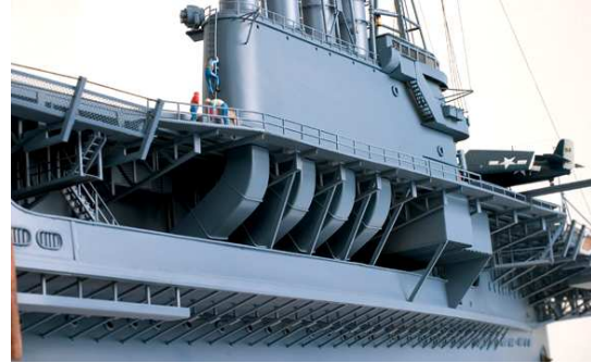
Figure 4 - Uptakes from boilers and island structure
