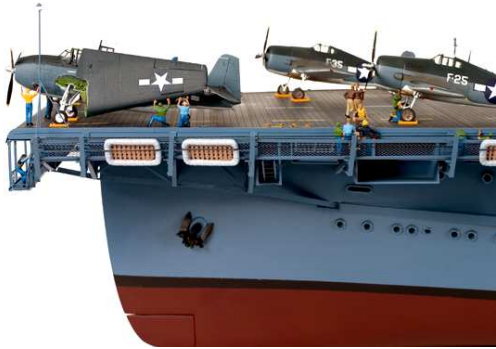
Figure 3- Bow, showing unique auxiliary rudder almost hidden in vessel's forefoot
